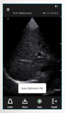
Enabled and disabled with longer keystroke on gain button.
